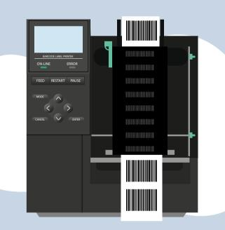
**Ribbon save technology** Ribbon save technology reduces costs, because the print head lifts up between barcodes, saving ribbon when using pre-printed labels
